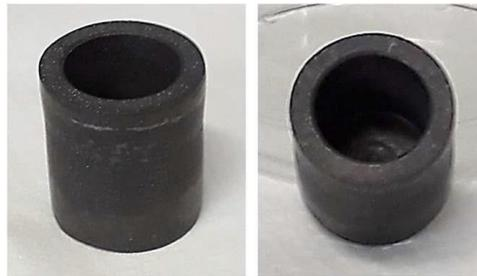
**Fig. 2** MgB<sub>2</sub> cup fabricated by spark plasma sintering, drilling and final refining on a lathe machine. Geometrical parameters: outer radius,  $R_o = 10.15$  mm, inner radius,  $R_i = 7.0$  mm, external height,  $h_e = 22.5$  mm, internal depth,
