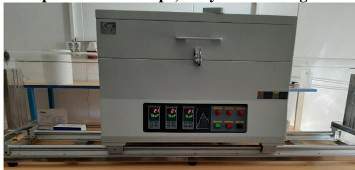
**Physical Vapor Transport equipment for transition metal dichalcogenides**
