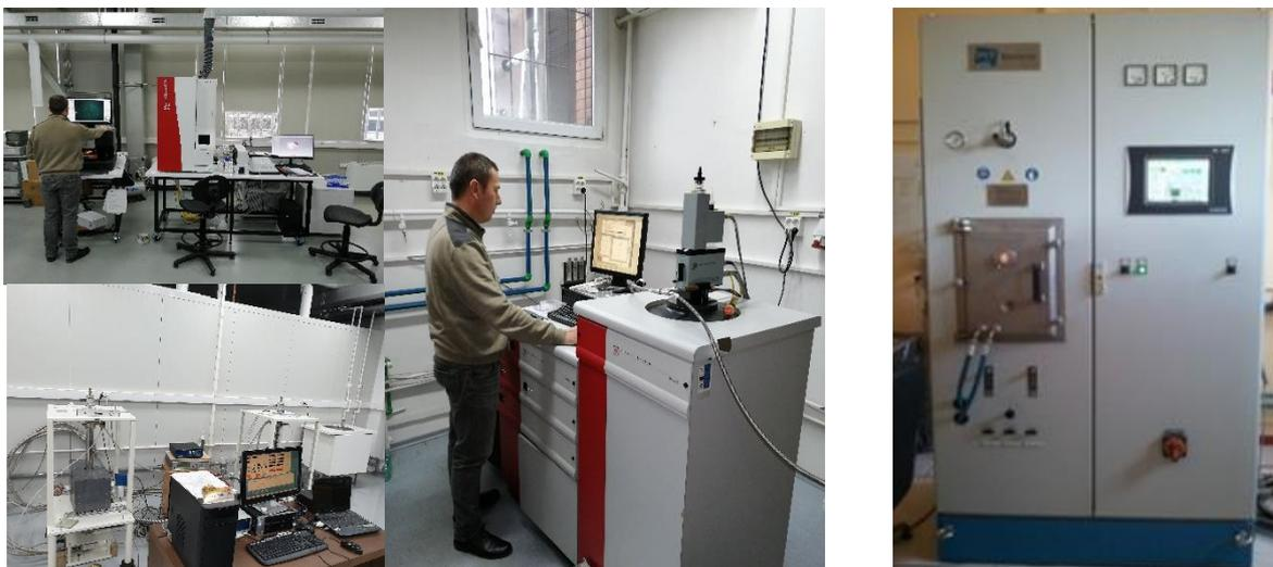
ICP-MS with LA for thin films (upper left), Mossbauer spectrometers with closed circuit He cryostats (lower left) and SQUID device – Quantum Design, of high sensitivity (middle). Spark plasma sintering plant (FCT Systeme GmbH) used to obtain high density bulk materials (right).
