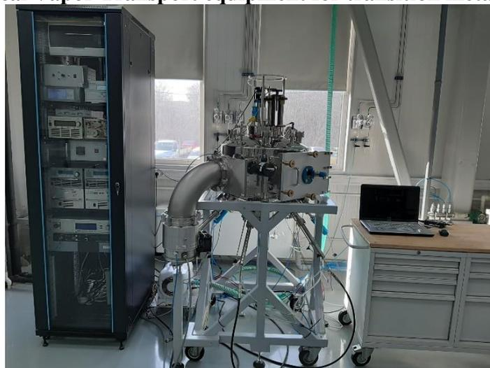
**Hybrid Magnetron Sputtering – Pulsed Laser Deposition equipment for thin films**
